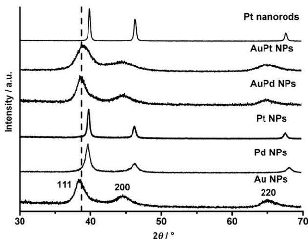
Figure 1. XRD patterns for noble-metal and alloy nanocrystals.
