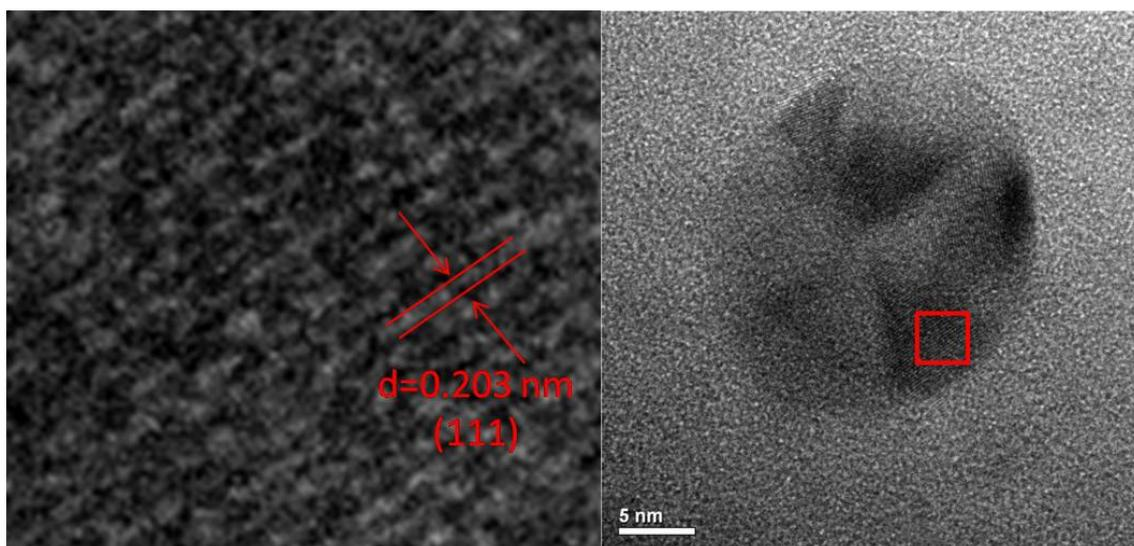
**Figure S1** High-magnification TEM images of nickel particles on 17% Ni/ZSM-5
