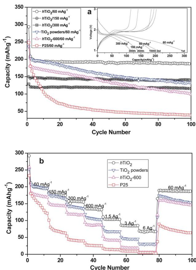
**Fig. 7** Comparative cycling performance of as-prepared TiO<sub>2</sub> samples (a) for 100 cycles and (b) at different current densities. The inset in (a) shows the typical charge–discharge voltage profiles of hTiO<sub>2</sub> nanoparticles.
