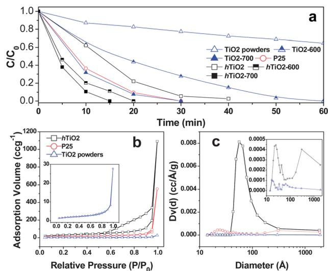
**Fig. 6** (a) Catalytic performance of the TiO<sub>2</sub> samples assessed by the photo-degradation of RhB. (b) Nitrogen adsorption-desorption isotherms and (c) pore size distribution of the TiO<sub>2</sub> samples. The inset in (b) shows an enlargement of TiO<sub>2</sub> powders and the inset in (c) shows an enlargement of TiO<sub>2</sub> powders and P25.
