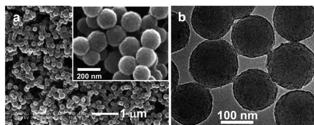
**Fig. 2** (a and b) SEM and TEM images of  $\text{C@Ti}(\text{OH})_4$  particles.
