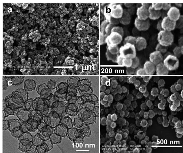
**Fig. 5** (a–c) SEM and TEM images of hollow TiO<sub>2</sub> nanoparticles. (d) SEM photograph of aggregated hollow TiO<sub>2</sub> nanoparticles.
