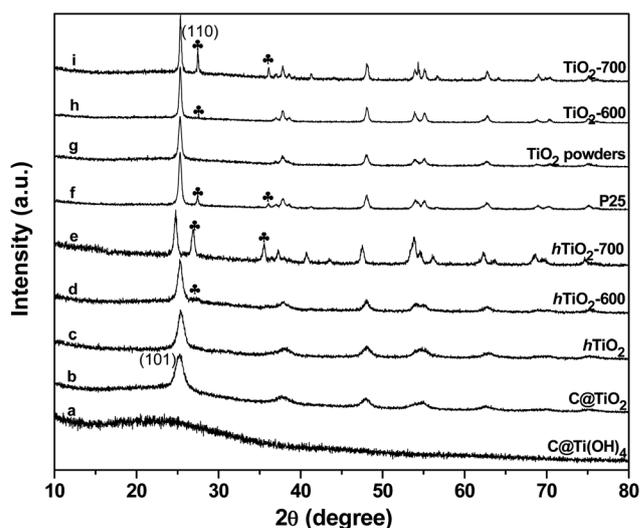
**Fig. 4** XRD patterns of as-prepared  $\text{TiO}_2$  samples prepared under different conditions.
