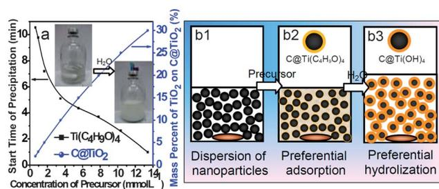
**Fig. 1** (a) Start time of precipitation and the mass percent of  $\text{TiO}_2$  on  $\text{C@TiO}_2$  particles as functions of the concentration of the precursors in ethanol. The picture in the inset shows the equipment used for the reaction. (b1–b3) Schematic drawing of the coating process.
