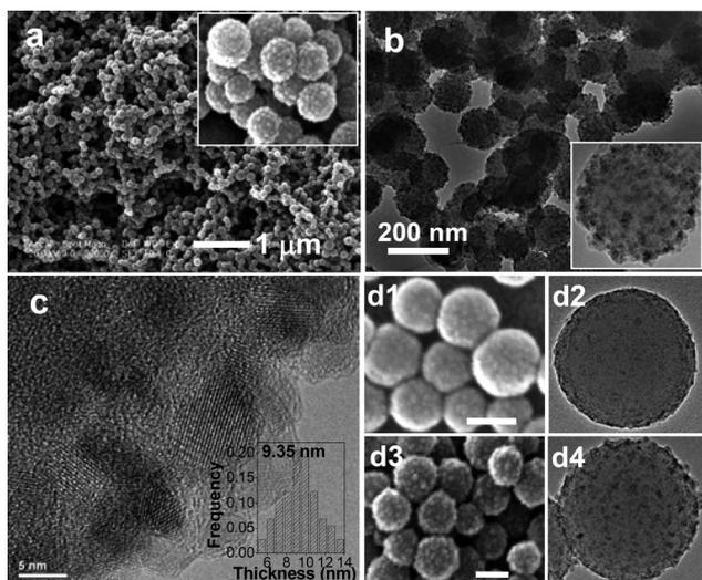
**Fig. 3** (a–c) SEM, TEM, and HRTEM images of  $\text{C@TiO}_2$  particles with a  $\text{TiO}_2$  loading of 30%. (d1–d4) SEM and TEM images of  $\text{TiO}_2/\text{C}$  and  $\text{C@TiO}_2$  particles with 5 wt% and 20 wt%  $\text{TiO}_2$ . The unlabelled scale bar is 100 nm.
