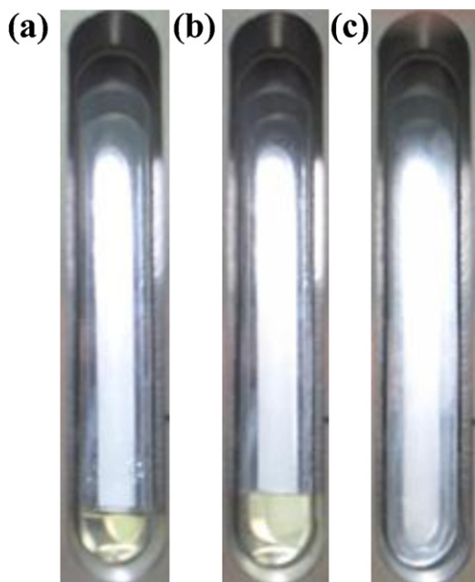
Fig. 3. Visual observations of the reaction mixture including o -CNB, H 2 , and CO 2 at 35 °C and at CO 2 pressure given (a) 0.1 MPa, (b) 9 MPa, (c) 17.4 MPa. Conditions: viewing cell volume 74 ml, 2.22 g o -CNB, 4 MPa H 2 .
