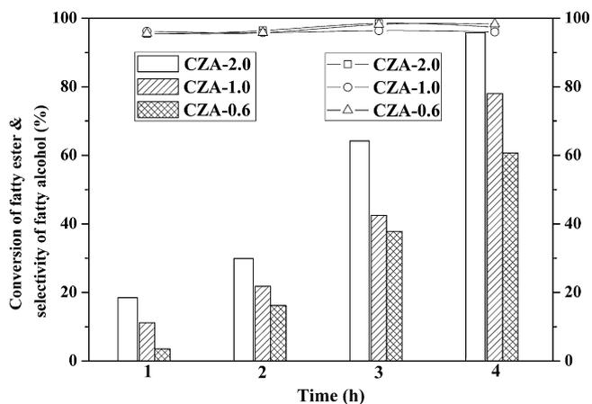
**Fig. 3.** A plot of the conversion (column) and selectivity (line) against the reaction time over CuO/ZnO/Al<sub>2</sub>O<sub>3</sub> catalysts. Reaction conditions: ethyl stearate 1.0 mmol, catalyst 50 mg, hexane 5.0 ml, H<sub>2</sub> 3.0 MPa, 230 °C.
