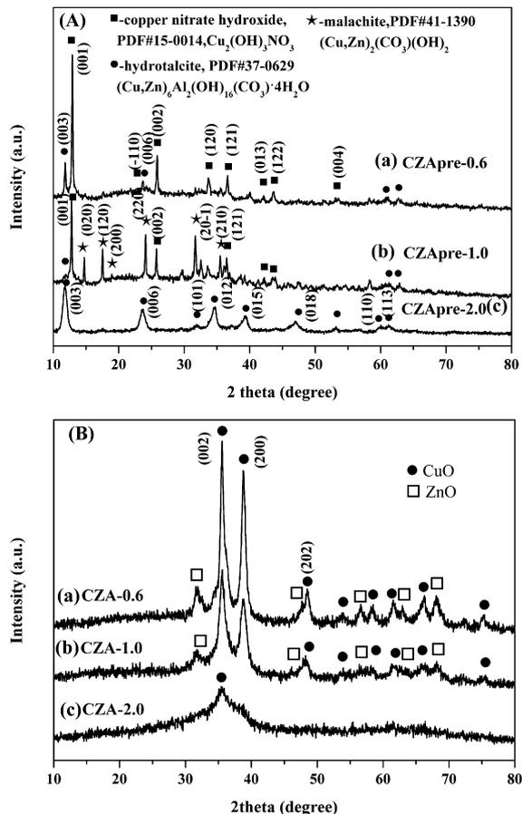
**Fig. 1.** The XRD patterns of catalysts precursors (A) prepared at alkali concentration of (a) 0.6 M, (b) 1.0 M, and (c) 2.0 M; and (B) catalysts calcined at 350 °C (3 h).
