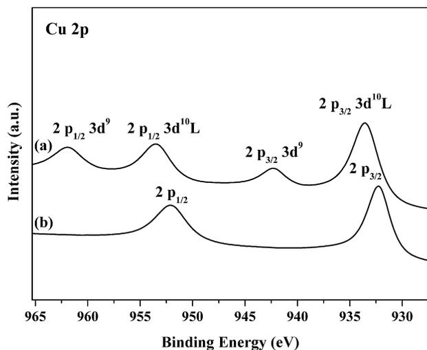
Fig. 5. XPS spectra of CZA-2.0. (a) Fresh catalyst and (b) used catalyst.
