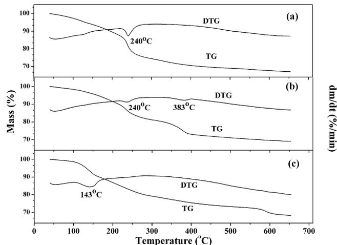
**Fig. 2.** TG–DTG curves of the precursors. (a) CZApré-0.6, (b) CZApré-1.0, and (c) CZApré-2.0.
