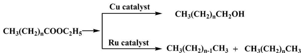
**Scheme 1.** Hydrogenation reaction route of aliphatic fatty ester ( $n = 16$  for ethyl stearate).
