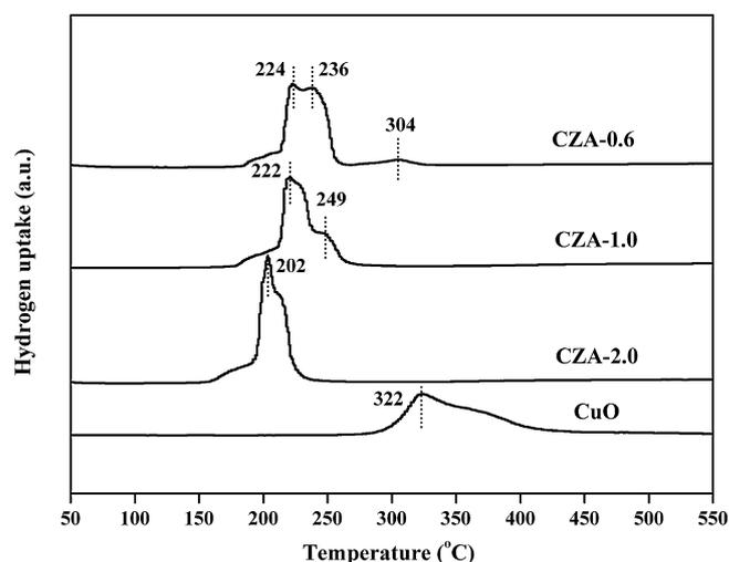
**Fig. 4.** TPR profiles of the catalyst prepared at different concentration of alkali.
