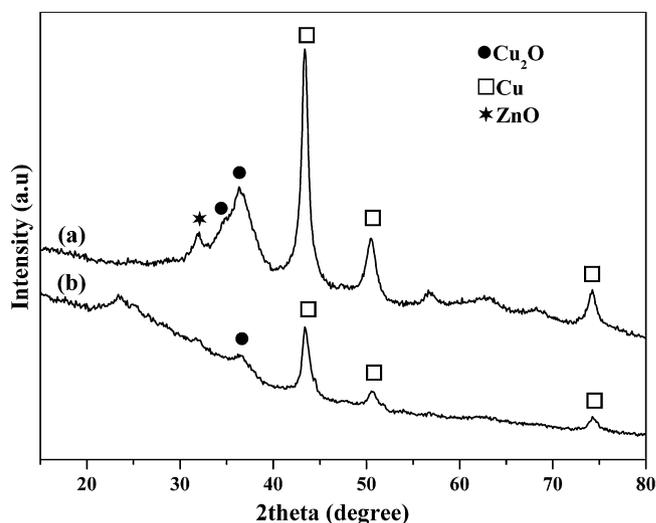
Fig. 6. The XRD patterns of CZA-2.0. (a) Used catalyst and (b) reduced catalyst.
