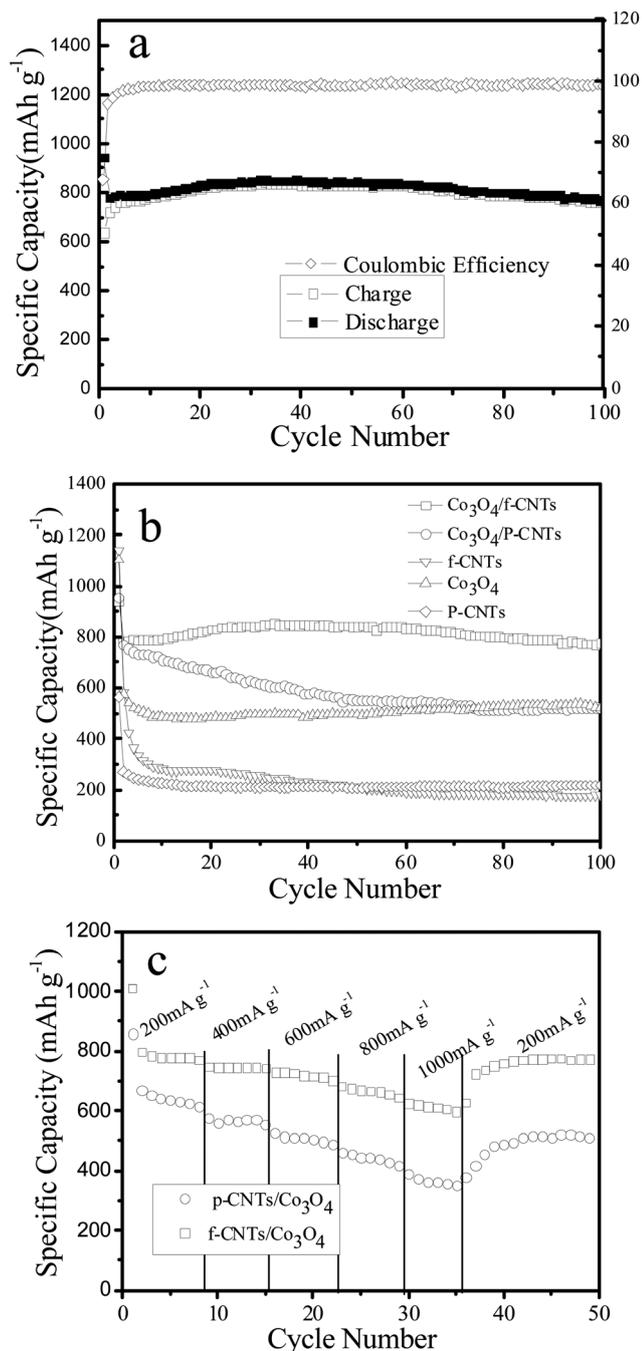
**Fig. 7** (a) Cycling behaviour of the Co<sub>3</sub>O<sub>4</sub>-f-CNT composite at a current density of 200 mA g<sup>-1</sup>. (b) Cycling behaviours of Co<sub>3</sub>O<sub>4</sub>-f-CNT, Co<sub>3</sub>O<sub>4</sub>-p-CNT, f-CNTs, p-CNTs, and Co<sub>3</sub>O<sub>4</sub> (commercial) at a current density of 200 mA g<sup>-1</sup>. (c) Discharge capacity vs. cycle number of Co<sub>3</sub>O<sub>4</sub>-f-CNT and Co<sub>3</sub>O<sub>4</sub>-p-CNT composite electrodes at various current densities.
