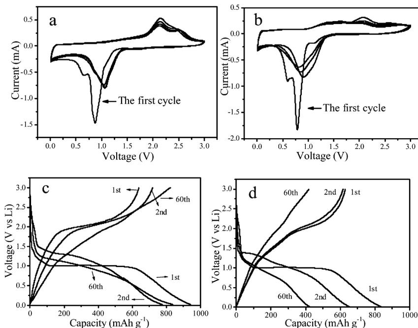
**Fig. 6** Typical cyclic voltammograms of (a)  $\text{Co}_3\text{O}_4$ -f-CNT and (b)  $\text{Co}_3\text{O}_4$ -p-CNT at a sweep rate of  $0.2 \text{ mV s}^{-1}$ . The 1<sup>st</sup>, 2<sup>nd</sup>, and 60<sup>th</sup> charge–discharge voltage profiles of  $\text{Co}_3\text{O}_4$ -f-CNT (c) and  $\text{Co}_3\text{O}_4$ -p-CNT composite electrodes (d) at a current density of  $200 \text{ mA g}^{-1}$ .
