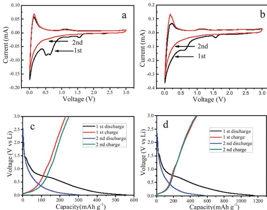
**Fig. 5** Cyclic voltammograms (CVs) of p-CNTs (a) and f-CNTs electrodes (b) at a scan rate of  $0.2 \text{ mV s}^{-1}$  during the first two cycles. The first two charge–discharge voltage profiles of (c) p-CNTs and (d) f-CNTs.
